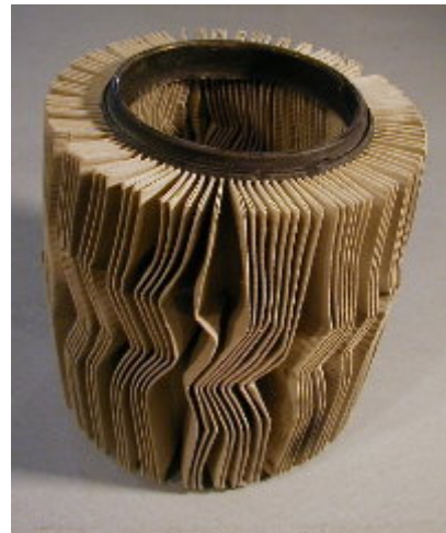
Sears Shop-Vac filter. Paper pleats. This filter has stood up for 12 years in my 8 gallon shop-vac.
