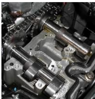
These cams are at TDC. The gear that I removed is bolted lightly to the cam already.
